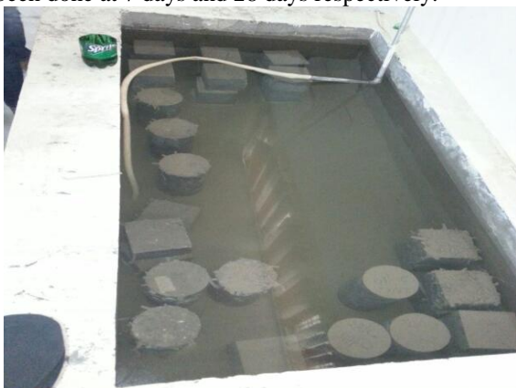
Fig 2: Plastic Fiber Cement Concrete Cubes Curing
