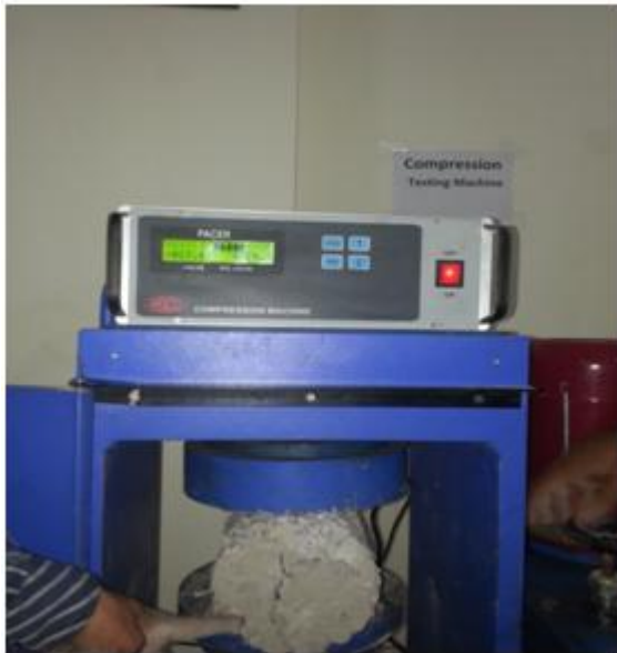
Fig 6: 28 days split tensile strength
